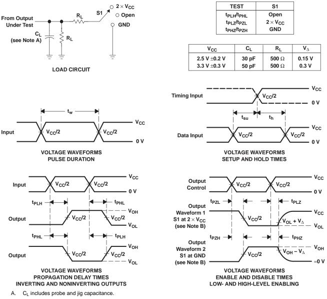
B. Waveform 1 is for an output with internal conditions such that the output is low, except when disabled by the output control.
