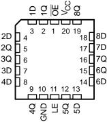
OE does not affect the internal operations of the latches. Old data can be retained or new data can be entered while the outputs are in the high-impedance state.
