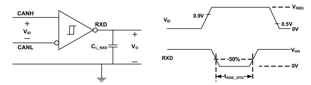
Figure 8. RXD Dominant Timeout Test Circuit and Measurement
