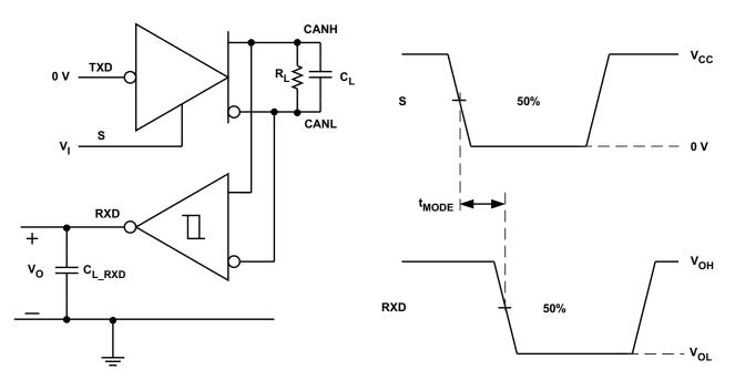
Figure 12.  $t_{\text{MODE}}$  Test Circuit and Measurement
