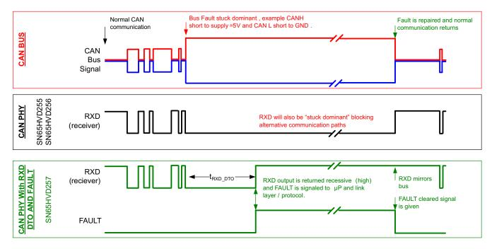
Figure 7. Example Timing Diagram for Devices With and Without RXD DTO and FAULT Pin
