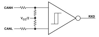
Figure 4. Simplified Recessive Common Mode Bias and Receiver
