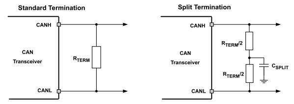
Figure 19. CAN Bus Termination Concepts
