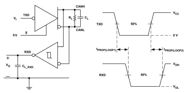
Figure 13. T<sub>PROP(LOOP)</sub> Test Circuit and Measurement
