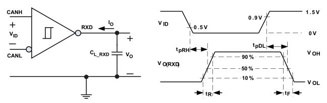
Figure 11. Receiver Test Circuit and Measurement
