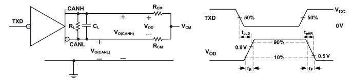
Figure 10. Driver Test Circuit and Measurement
