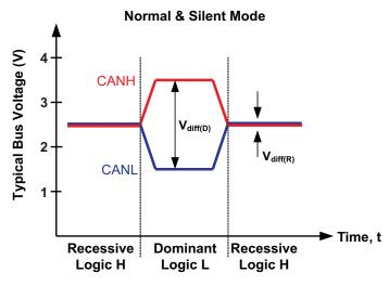
Figure 3. Bus States (Physical Bit Representation)
