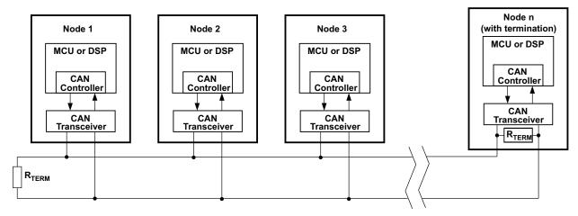
Figure 18. Typical CAN Bus
