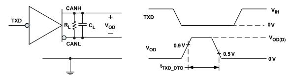
Figure 14. TXD Dominant Timeout Test Circuit and Measurement
