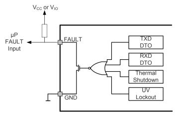
Figure 5. FAULT Pin Function Diagram and Application
