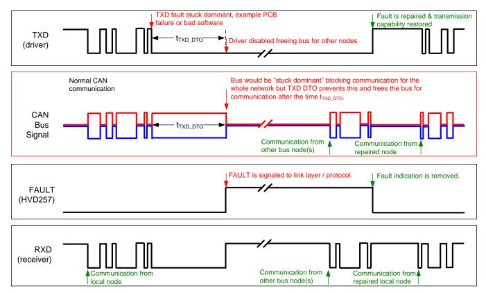
Figure 6. Example Timing Diagram for TXD DTO and FAULT Pin
