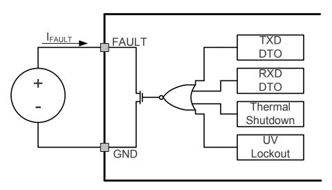
Figure 9. FAULT Test and Measurement
