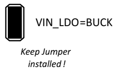
Figure 4. VIN_LDO=BUCK Jumper Setting
