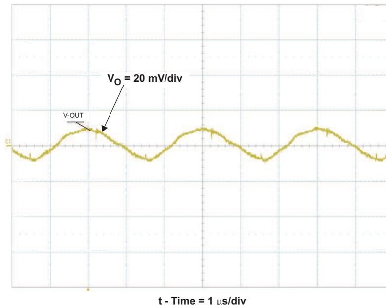
Figure 6. TPS55010EVM-009 Output Voltage Ripple
