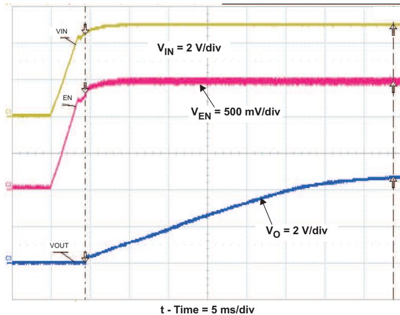
Figure 8. TPS55010EVM-009 Start-Up With Rising  $V_{IN}$
