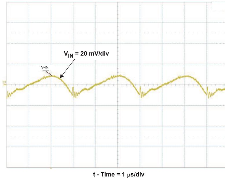
Figure 7. TPS55010EVM-009 Input Voltage Ripple
