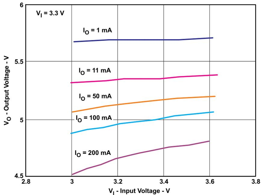
Figure 4. TPS55010EVM-009 Line Regulation, VIN = 3.3 V
