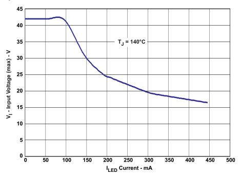
Figure 5. TL4242EVM-543 Maximum Vin vs LED Current
