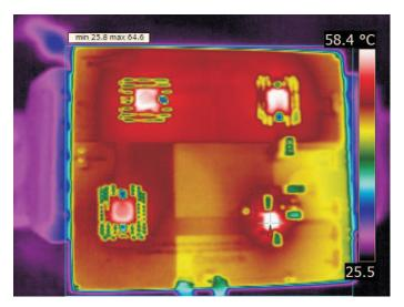
Figure 6. TL4242EVM-543 Top Infrared at  $V_{in}$  = 12 V,  $I_{LED}$  = 357 mA (Viewed From Top)
