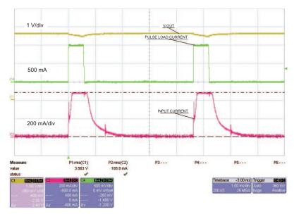
Figure 5. C4 Added 47  $\mu\text{F},$  1-A Pulse Load With Current Limit Set to High, Pulse 577  $\mu\text{s}$  at 216 Hz, Time Base 1 ms
