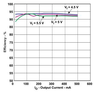
Figure 7. Efficiency With Current Limit Set to High, Vin 5 V, 4.5 V, and 5.5 V
