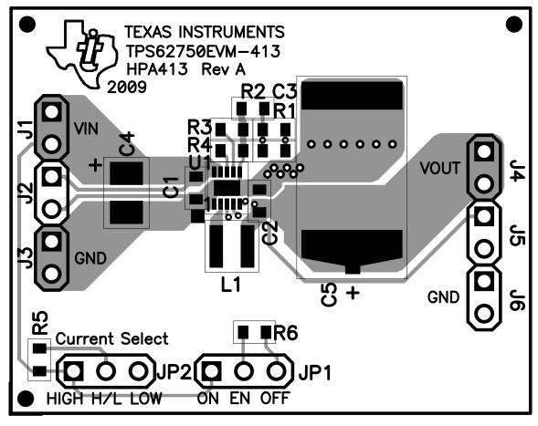
Figure 8. Top Assembly Layer
