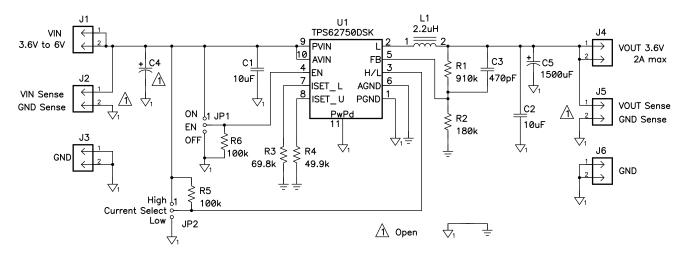
Figure 11. TPS62750EVM-413 Schematic
