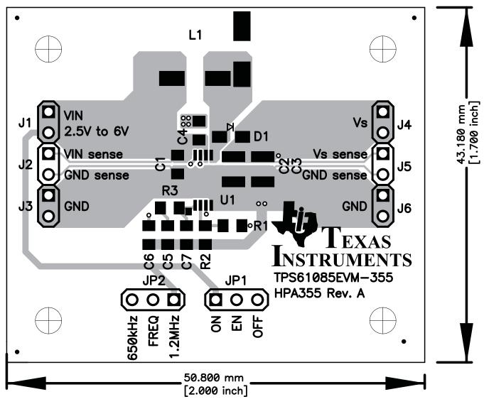
Figure 2. Top Assembly Layer
