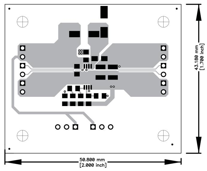
Figure 3. Top Layer Routing
