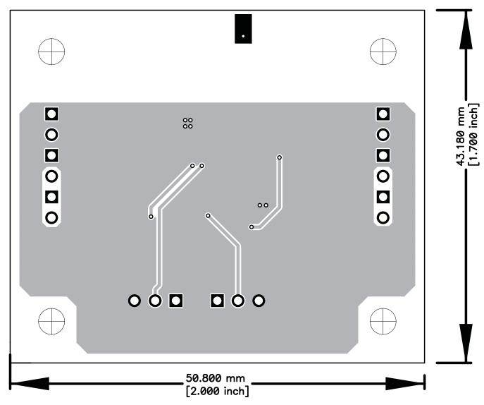
Figure 4. Bottom View of EVM Layer Routing
