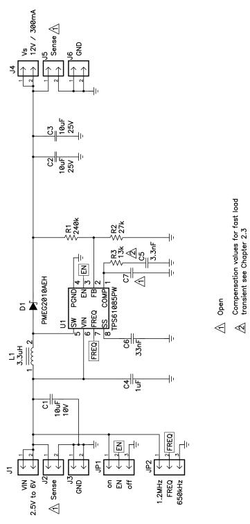
Figure 1. TPS61085EVM Schematic
