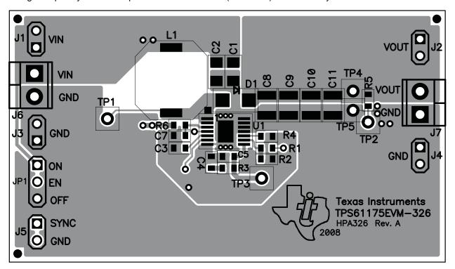
Figure 9. Top Assembly Layer
