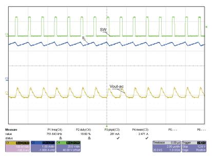
Figure 4. PWM Operation at 450 mA With  $V_{IN}$  = 5V
