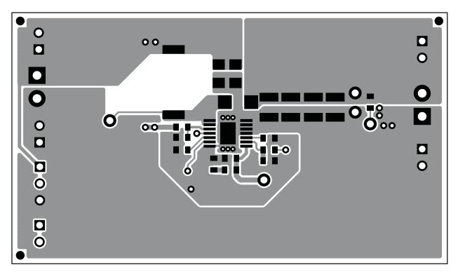
Figure 10. Top Layer Routing
