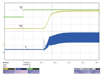
Figure 3. Start-Up With  $V_{\text{IN}}$  = 12V and  $I_{\text{OUT}}$  = 100 mA
