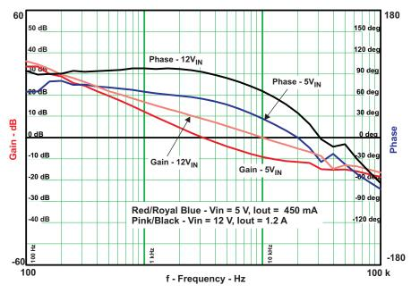
Figure 8. Loop Gain and Phase
