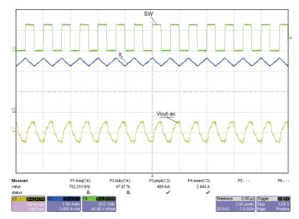
Figure 5. PWM Operation at 1.2 A With  $V_{IN}$  = 12V
