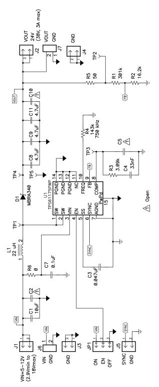
Figure 14. TPS61175EVM-326 Schematic
