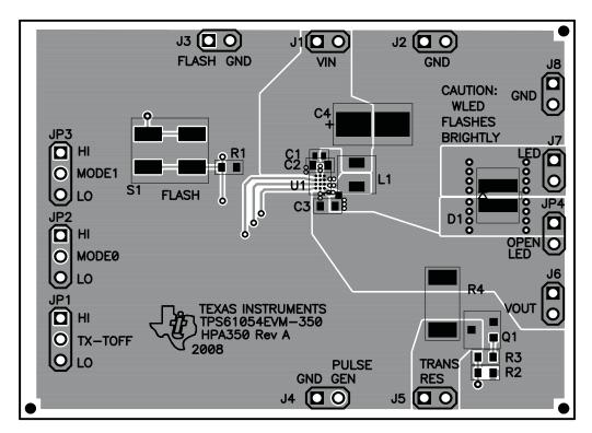
Figure 7. Assembly Layer
