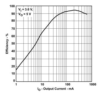
Figure 5. Voltage-Mode Efficiency
