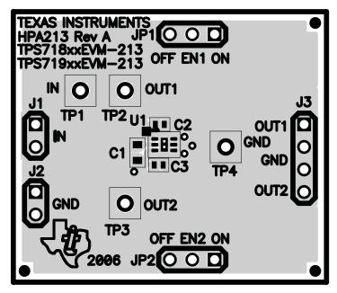
Figure 1. Assembly Layer
