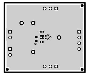
Figure 2. Top Layer Routing
