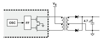
Figure 2. Simplified Transformer Driver
