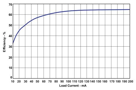
Figure 4. Efficiency Over Load Current
