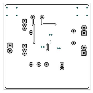
Figure 5. Bottom Copper (top view)
