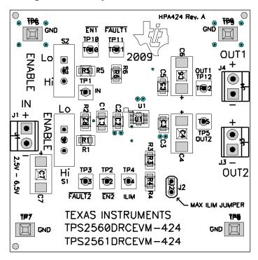
Figure 3. Top Layer Assembly (top view)
