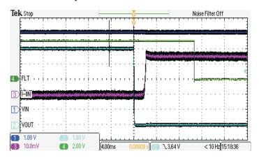
Figure 2. 100-k $\Omega$  R<sub>ILIM</sub> Enabled into a Short Circuit
