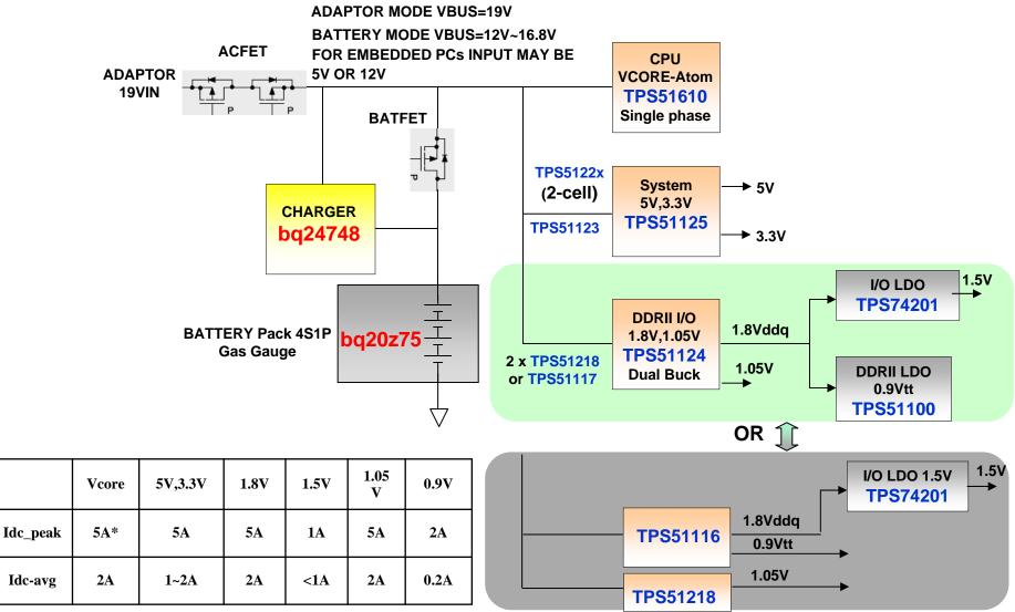
\*typical value measured from actual system & I/O LDO can be replaced by single PWM switcher.
