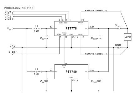
**External Capacitors:** When used with a PT7778, the PT7740 requires a minimum ouput capacitance of 330µE. The maximum allowable output capacitance is 30,000µE. The PT7740 also requires a minimum input capacitance of 2400µE, which must be rated for a minimum of 2.0Arms of ripple current. For transient or dynamic load applications, additional capacitance may be required. For further information, see the accompanying application note on capacitor selection for this product.
