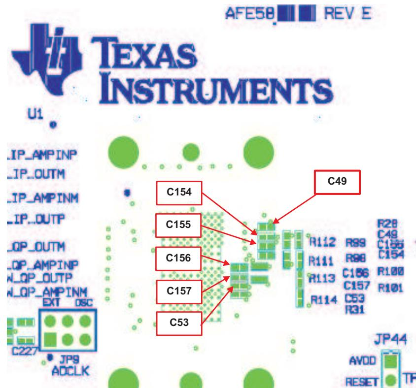
**Figure 7. Relevant Capacitors for CW Mode, Top Side**
