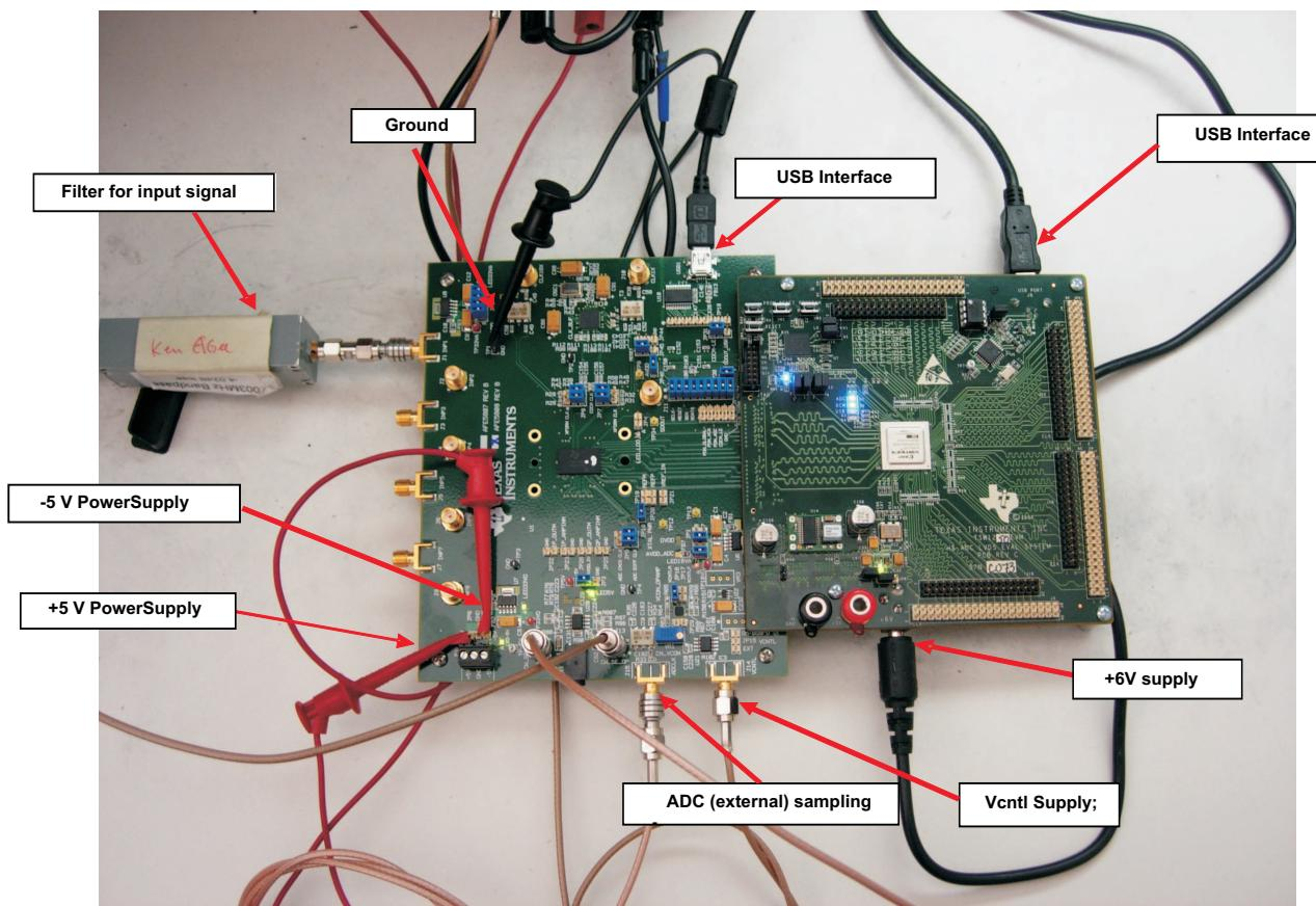
**Figure 2. HW Setup With Connection Between TSW1250EVM and AFE5807**
