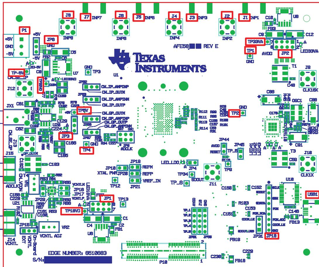
**Figure 11. I/O, PWR, and USB Connector**
