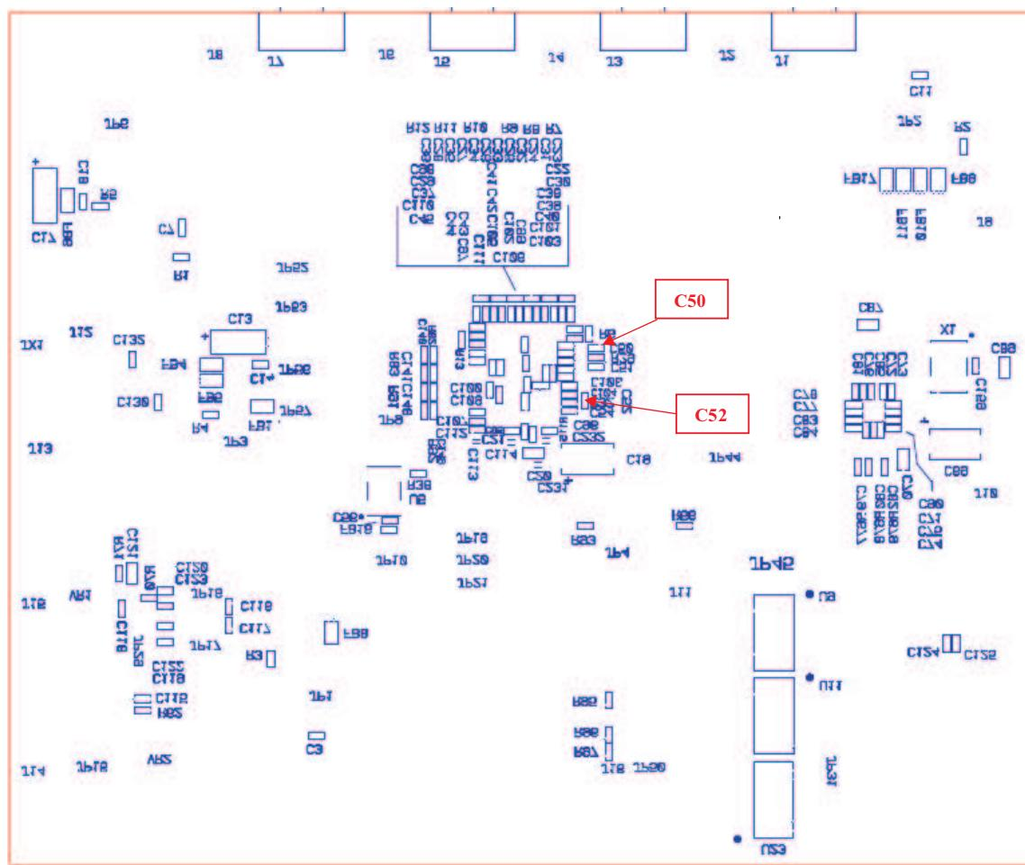
**Figure 8. Relevant Capacitors for CW Mode, Bottom Side**
