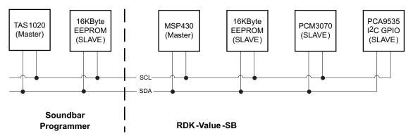
In a typical final product, the Soundbar Programmer board is not attached. It is only be used for development, and potentially, production line programming. The power supply on the RDK-Value-SB actually powers the TAS1020 streaming controller on the RDK-Value-SB. As such, the 3V3 regulator on the soundbar may dissipate a little more heat in development than in final use.
