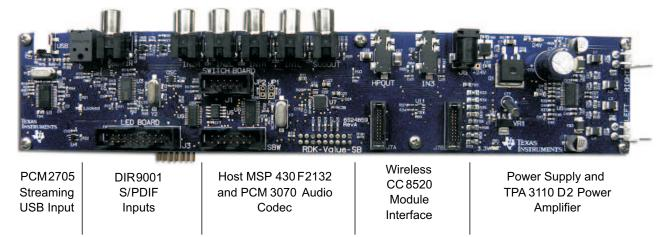
The core converter and processor in this reference design is the PCM3070 codec. The reference design takes advantage of the two different outputs available on the PCM3070: namely, the main DAC output and the I<sup>2</sup>S output to provide up to four different signal outputs. This allows systems with additional wireless subwoofers or extra DAC pairs to be added easily on dedicated headers on the printed-circuit board (PCB).
