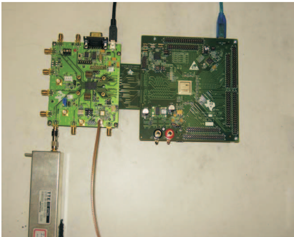
Figure 20. Connection between TSW1250EVM and AFE5805
