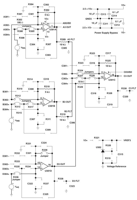
Figure 3–7. Quad Operational Amplifier Instrumentation Amplifier With Dual Supply Using Area 300
