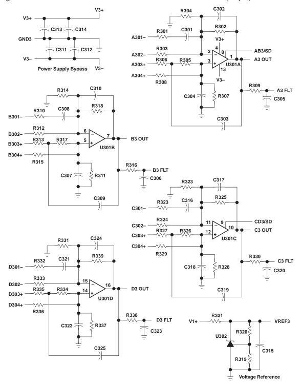
Figure 2–3. Area 300 Schematic—Quad Device TSSOP PowerPAD (16 pin)
