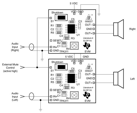
**Note:** The SE/BTL\* (SE/BTL) EVM pin is pulled to GND through a 100-KΩ resistor on the module.
