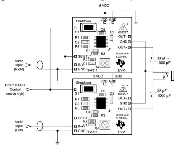
Figure 3–9. TPA311 EVM Connected for Stereo Single-Ended Output
