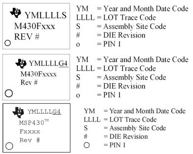
Note: Package marking with "TM" applies only to devices released after 2011.
