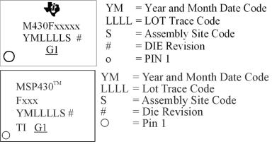
Note: Package marking with "TM" applies only to devices released after 2011.
