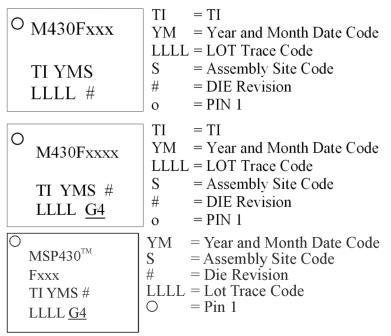
Note: Package marking with "TM" applies only to devices released after 2011.
