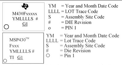
Note: Package marking with "TM" applies only to devices released after 2011.
