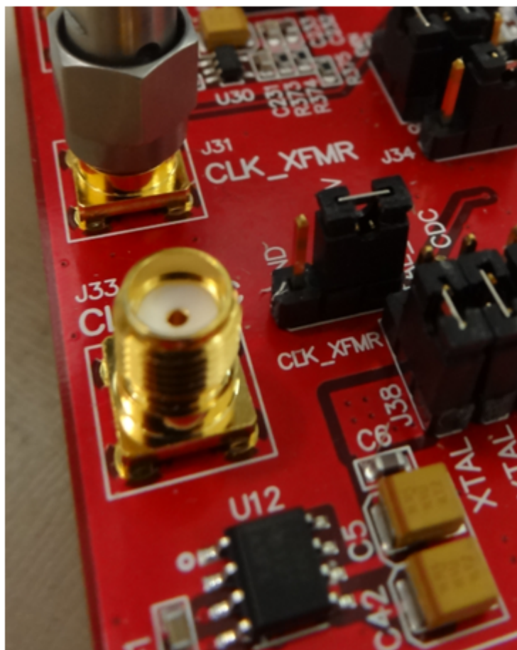
Figure 36. Jumper J35 and J38 positions for Enabled XTAL (default)
