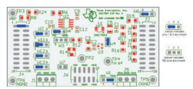
Figure 7. Factory Default Jumper Setting
