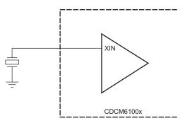
Note: This configuration assumes that the crystal is placed very closed to the XIN pin on the device.
