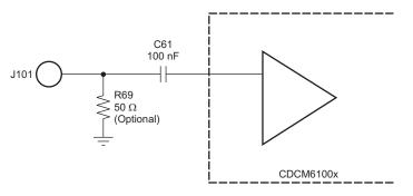
Figure 3. Single-Ended Connection Configuration
