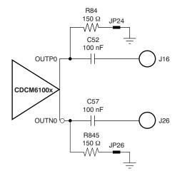
Figure 5. LVPECL Output Setup
