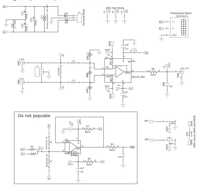
Figure 5. INA149EVM Complete Schematic
