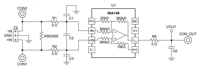
Figure 2. INA149EVM Input/Output Schematic
