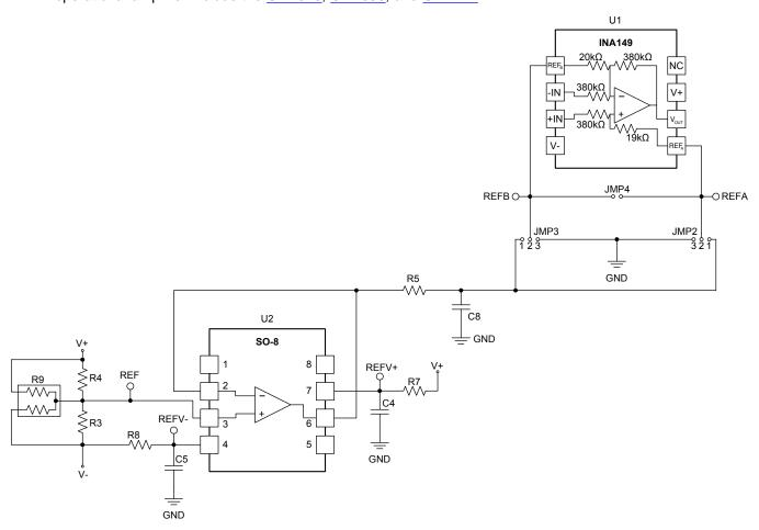
Figure 3. INA149EVM Reference Voltage Schematic
