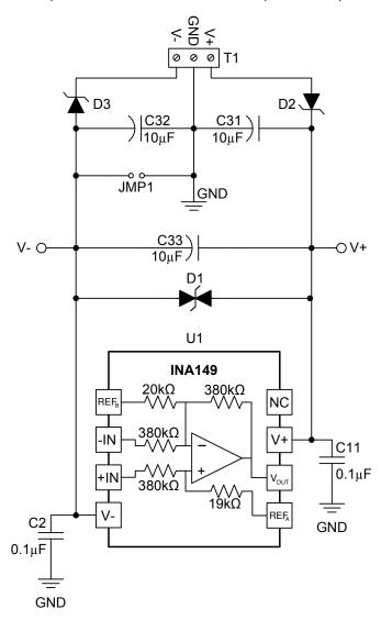
Figure 4. INA149EVM Power Schematic
