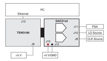
Figure 2. DAC31x2EVM Test Setup
