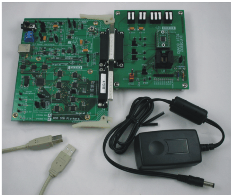
Figure 1. Hardware Included with the BUF08832EVM Kit
