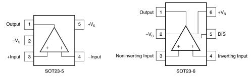
Figure 1. SOT23 Package Pinout, Top View
