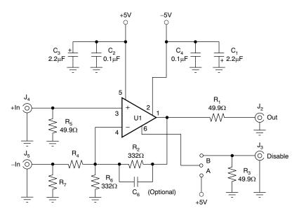
NOTE: Values for G = +2, OPA658.  $R_3$ ,  $R_4$ ,  $R_7$ ,  $C_5$  not assembled.
