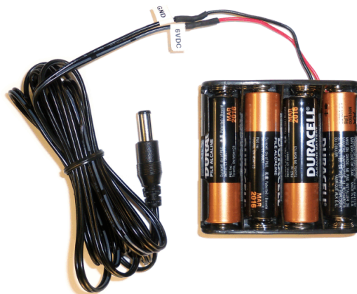
Figure 49. Recommended Power Supply for ADS1x98ECG-FE
