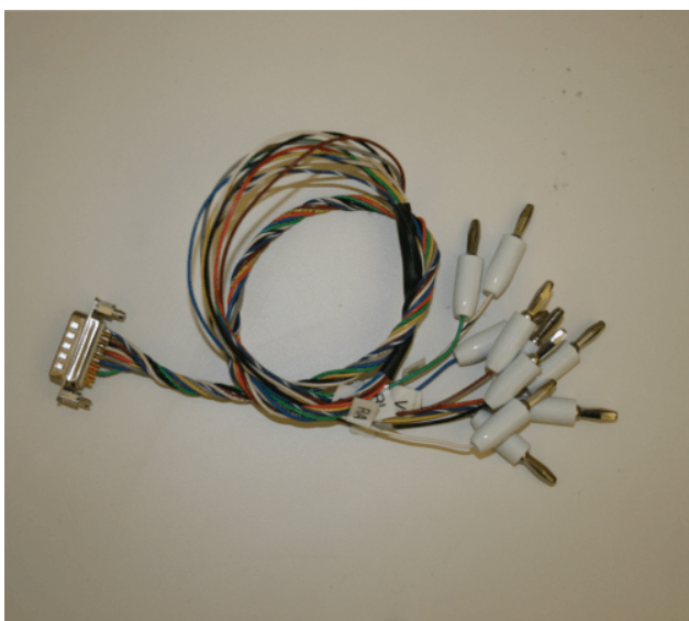
Figure 46. 15-Pin, Twisted Wire Cable to Banana Jacks
