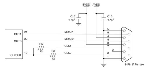
Figure 2. Power and Digital Outputs
