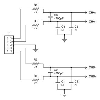
Figure 1. ADS1209EVM Schematic: Analog Input Section
