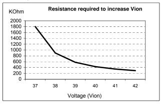
To increase Vion the resistor should be connected between pins 11 and 17.
