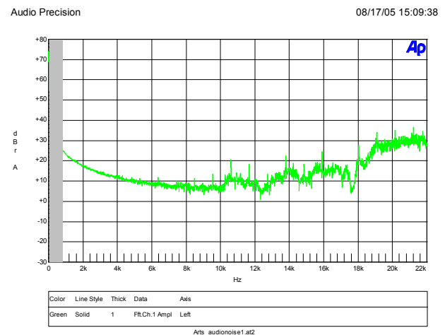
Figure 32 – Audible Noise V_{IN} = 230 \text{ VAC} ; I_{OUT} = 1.2 \text{ A} .
