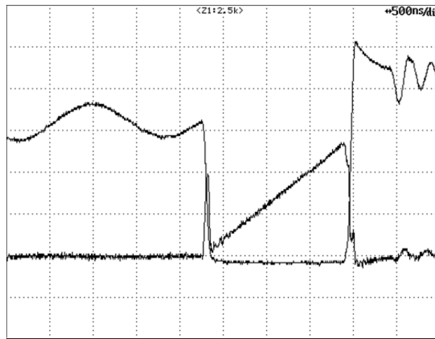
Figure 13 – 230 VAC, Full Load. Upper: I_{DRAIN} , 0.2 A / div. Lower: V_{DRAIN} , 100 V / div.
