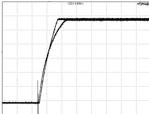
Figure 17 – Start-Up Profile, 230 VAC. Fast trace is no-load rise time. Slower trace is maximum load (12 \Omega ) 2 V, 5 ms / div.
