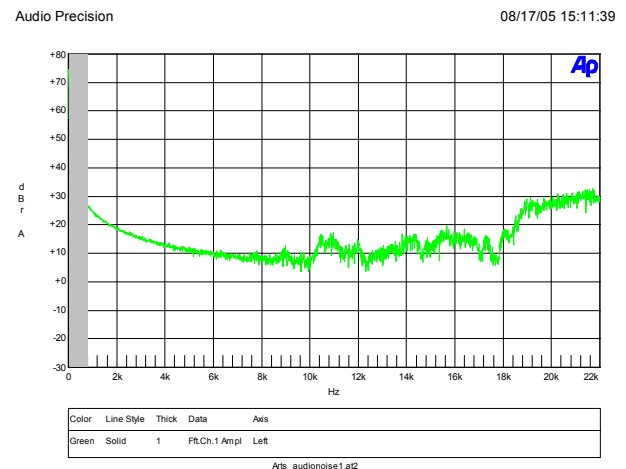
Figure 30 – Audible Noise V_{IN} = 120 \text{ VAC} ; I_{OUT} = 1 \text{ A} .
