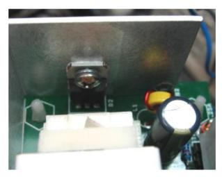
Figure 55 - Visible Light Output Rectifier Front View.
