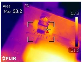
**Figure 58 –** Full Load HiperLCS Thermal View, Room Temperature.
