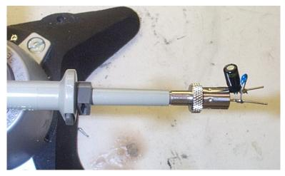
Figure 46 - Oscilloscope Probe with Probe Master (<a href="www.probemaster.com">www.probemaster.com</a>) 4987A BNC Adapter. (Modified with Wires for Ripple Measurement, and Two Parallel Decoupling Capacitors added)
