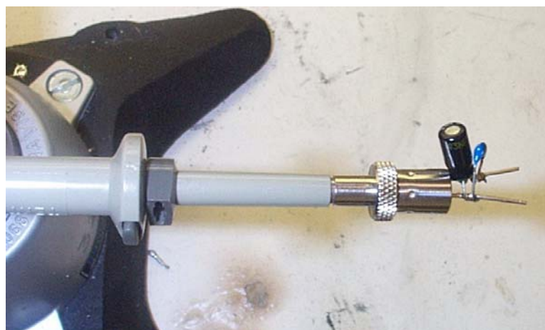
Figure 45 – Oscilloscope Probe with Probe Master 5125BA BNC Adapter. (Modified with wires for probe ground for ripple measurement, and two parallel decoupling capacitors added)
