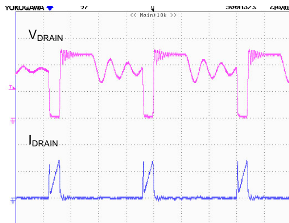
Figure 27 – 265 VAC, Full Load, -28 V Supply. Lower: I_{DRAIN} , 1 A / div. Upper: V_{DRAIN} , 200 V / div, 2 \mu s / div.
