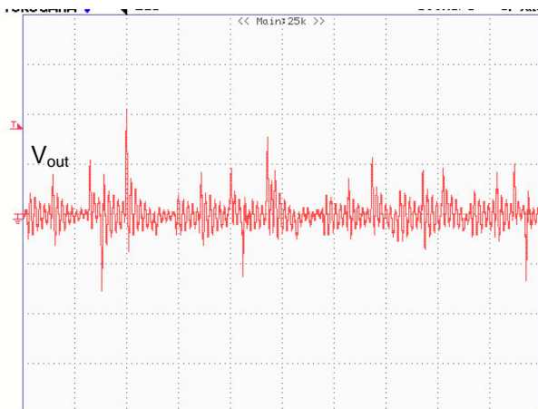
Figure 52 – +12 V Ripple, 90 VAC, 333 mA Load (889 mA on Main) 5 \mu s, 20 mV / div.
