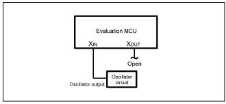
Figure 2.8 External oscillator circuit
