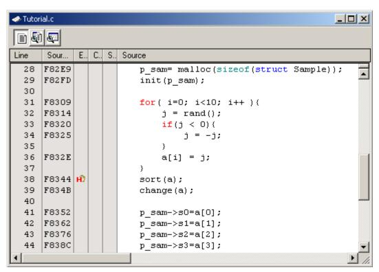
Figure 3.27 Editor window (setting a hardware breakpoint)
