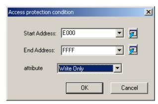
Figure 5.141 Access protection condition dialog box
