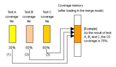
Figure 5.101 Schematic of merge-mode application
