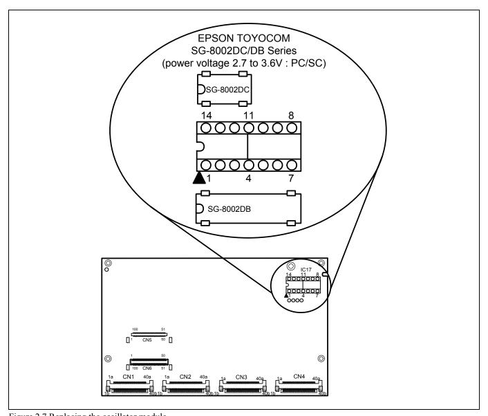
Figure 2.7 Replacing the oscillator module
