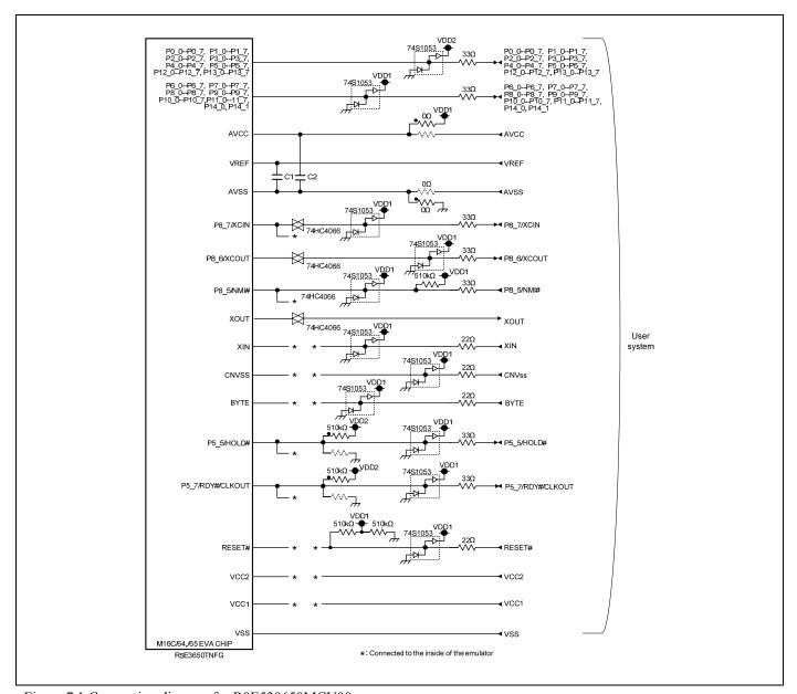
Figure 7.1 Connection diagram for R0E530650MCU00
