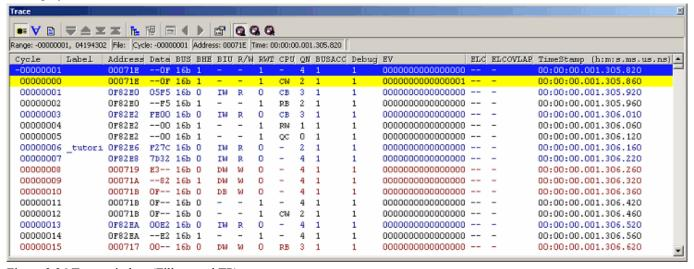
Figure 3.36 Trace window (Fill around TP)
