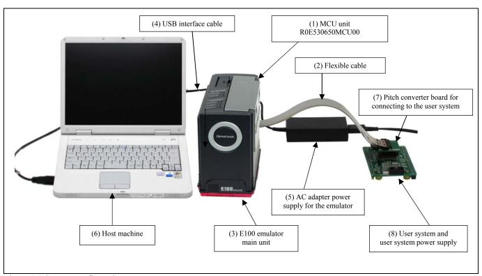
Figure 1.1 System configuration
