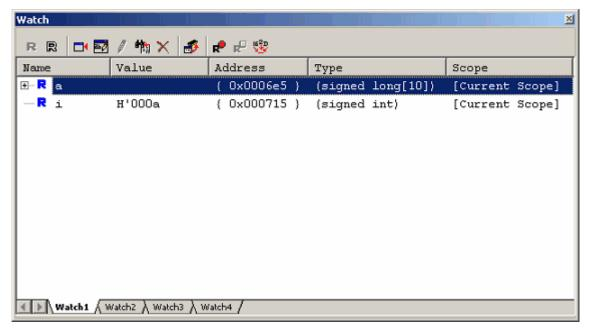
Figure 3.16 Watch window (showing a variable)
