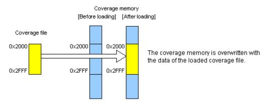
Figure 5.99 Schematic of the overwrite mode
