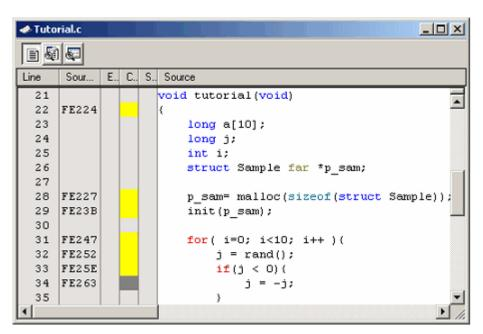
Figure 5.102 Example of code coverage results
