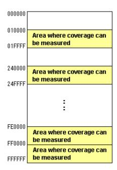
Figure 5.105 Schematic of data coverage memory allocation
