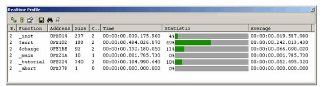
Figure 5.130 Realtime Profile window (function profile)
