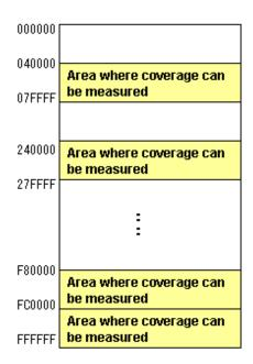
Figure 5.74 Schematic of coverage memory allocation
