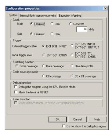
Figure 5.2 Configuration properties dialog box (System page)
