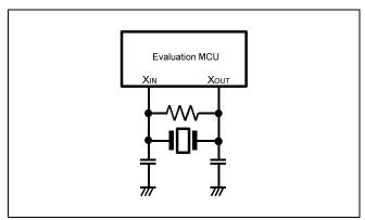
Figure 2.9 Circuit in which oscillation does not occur
