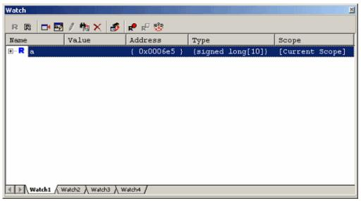
Figure 3.14 Watch window (array display)
