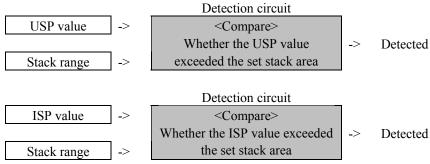
Figure 5.146 Outline of the detection of a stack access violation
