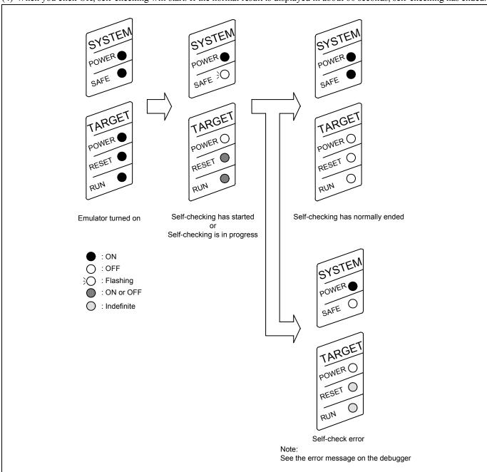
Figure 2.6 LED displays during the self-checking
