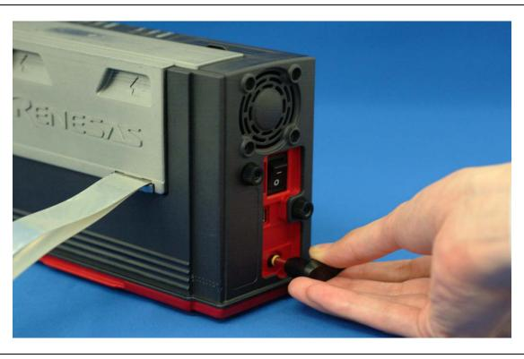
Figure 2.5 Connecting the emulator power supply
