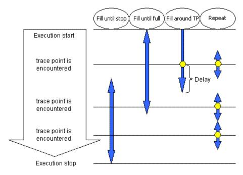
Figure 5.49 Differences between the trace modes
