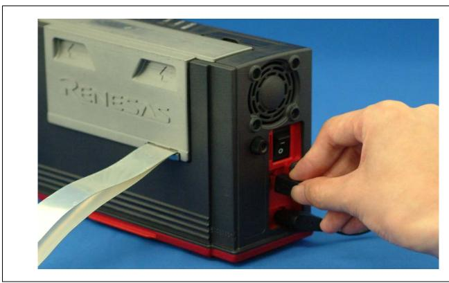
Figure 2.4 Connecting the host machine
