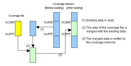
Figure 5.100 Schematic of the merge mode
