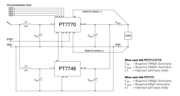
Output Capacitors: When used with a PT7771 or PT7772, the PT7746 requires a minimum ouput capacitance of 2400µE. When used with a PT7777, the PT7746 requires a minimum ouput capacitance of 680µE for proper operation. Do not use Oscon type capacitors. The maximum allowable output capacitance is 30,000µE.
