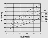
Note 1: All data listed in the above graphs, except for derating data, has been developed from actual products tested at 25°C. This data is considered typical data for the ISR. Note 2: Thermal derating graphs are developed in free air convection cooling of 40-60 LFM. (See Thermal Application Notes.)
