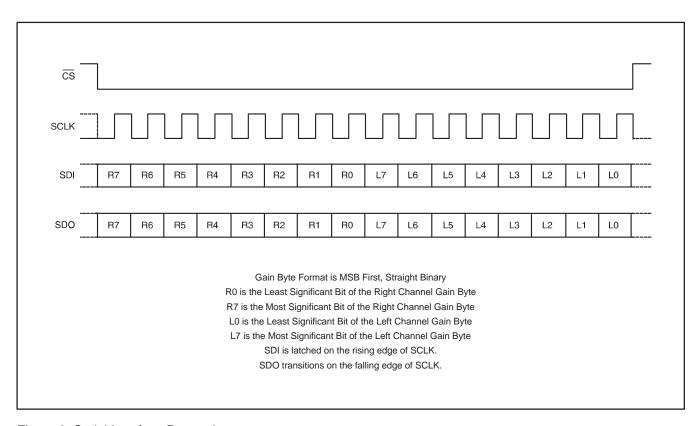
Figure 2. Serial Interface Protocol.
