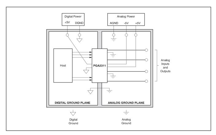
Figure 6. Typical PCB Layout Floor Plan.
