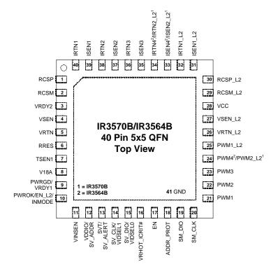
Figure 1: IR3564B/70B Pin Diagram Enlarged
