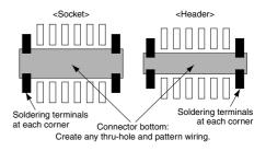
4. Gull-wing-shaped terminals to facilitate visual inspections.
