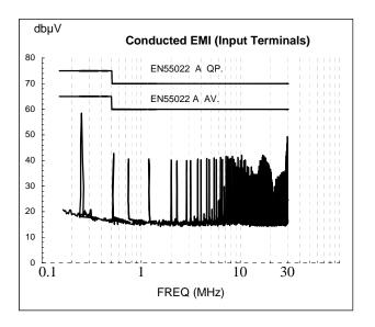
To meet class B for the above standards, it is necessary to fit a 3.3  $\mu F$  ceramic capacitor across the input terminals.
