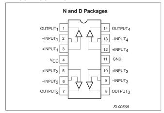
Figure 1. Pin configuration.
