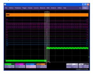
A second grid is created of the zoomed traces. Use either the Zoom control knobs (WaveRunner Xi, WavePro 7 Zi, WaveMaster 8 Zi, series) or the Vertical/Horizontal control knobs (WaveSurfer Xs Series) to adjust the vertical and horizontal scale and position. Reference your oscilloscope operator's manual for more information
