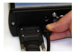
Connect the Digital Lead Set to the other end of the MS-250 (labeled Digital Inputs, D0 – D17) and fasten the thumb screws.
