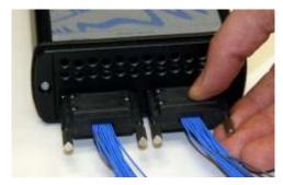
**NOTE**: Each digital line has a ground connection for optimal performance. Two additional ground leads common to the whole lead set are also available.
