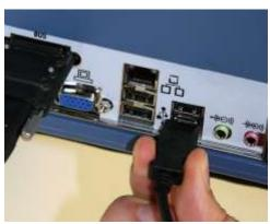
3. Connect the other end of the Teledyne LeCroy Bus cable to the MS-250 and fasten the thumb screws.
