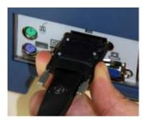
2. Connect the USB 2.0 cable (attached to the Teledyne LeCroy Bus cable) to any of the side mounted USB ports on the oscilloscope.
