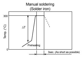
5-3. Recommended soldering peak temp and peak temp duration
