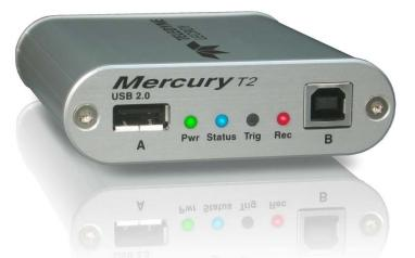
The Teledyne LeCroy Mercury™ T2 is the industry's smallest, most affordable hardware-based USB 2.0 protocol analyzer that combines the de-facto standard CATC Trace display with the very latest USB class decoding. The Mercury T2 fits in a shirt pocket yet provides much of the same lab quality protocol analysis capabilities offered in Teledyne LeCroy's top-of-the-line USB analyzers.
