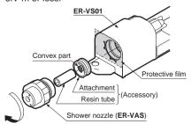
Note: Be sure to fit the resin tube and the attachment When they are not fitted, the static removal capability remarkably deteriorates.
