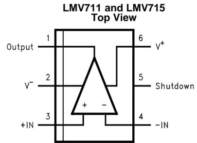
**Figure 47. 6-Pin SOT-23 Package
