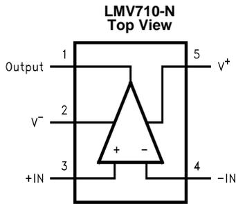
**Figure 46. 5-Pin SOT-23 Package
