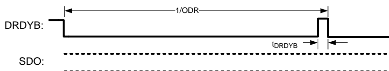
Figure 53. DRDYB Behavior for an ADC_DOUT not Read
