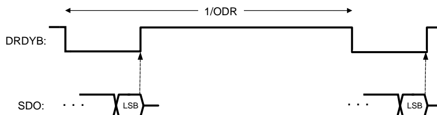
Figure 52. DRDYB Behavior for a Complete ADC_DOUT Reading
